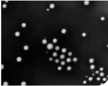
TEM of PLGA-Nanoparticles with a mean diameter of 140nm.
