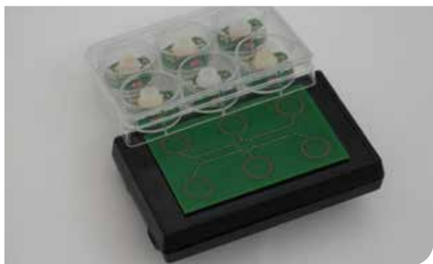
Sensor tags in a 6-well microtiter plate and a NFC reader system for energy and data transfer
